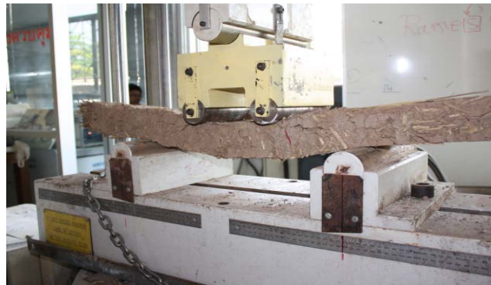
Figure 6 Complete test set up for third point load test in accordance with ASTM C 78-94
